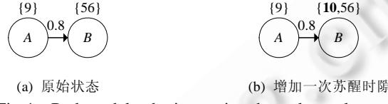
Fig.4 Reduce delay by increasing the wakeup slot
