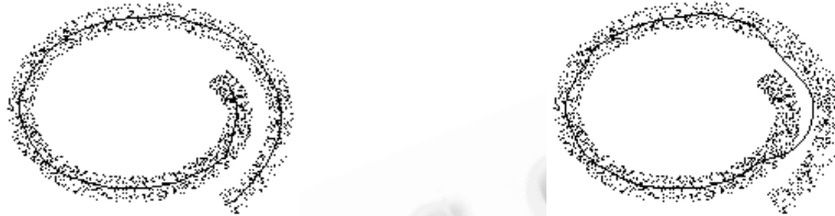
(a) Curve reconstructed by minimum spanning tree (b) Curve reconstructed without minimum spanning tree (a) 采用最小生成树的重建曲线 (b) 未采用最小生成树的重建曲线
