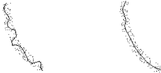
(a) Curve reconstructed without fairness term (b) Curve reconstructed with a fairness term (a) 未含光顺项的重建曲线 (b) 含光顺项的重建曲线
