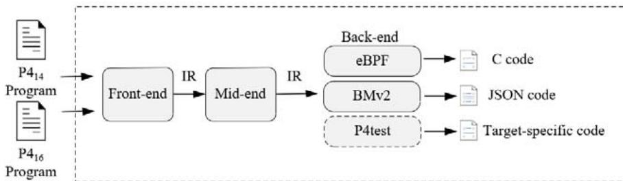
Fig.3 P4 program compilation process diagram
