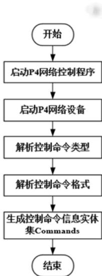
Fig.5 Control command parsing flowchart
