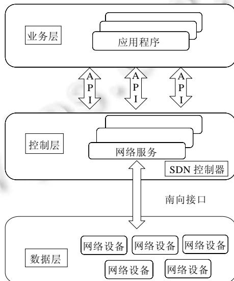
Fig.1 SDN network architecture
