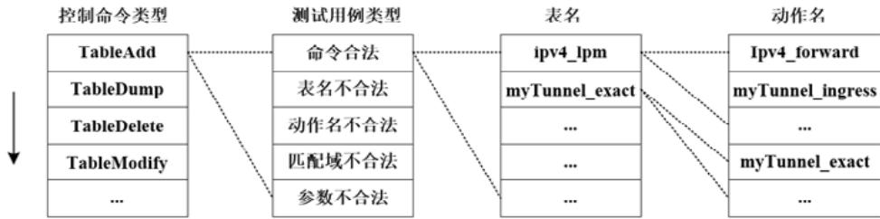
Fig.12 SDN data plane software conformance test case generation algorithm map for P4 programming language
