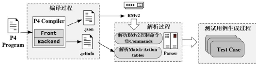
Fig.2 SDN data plane software conformance testcase generation tool data flow diagram for P4 programming language
