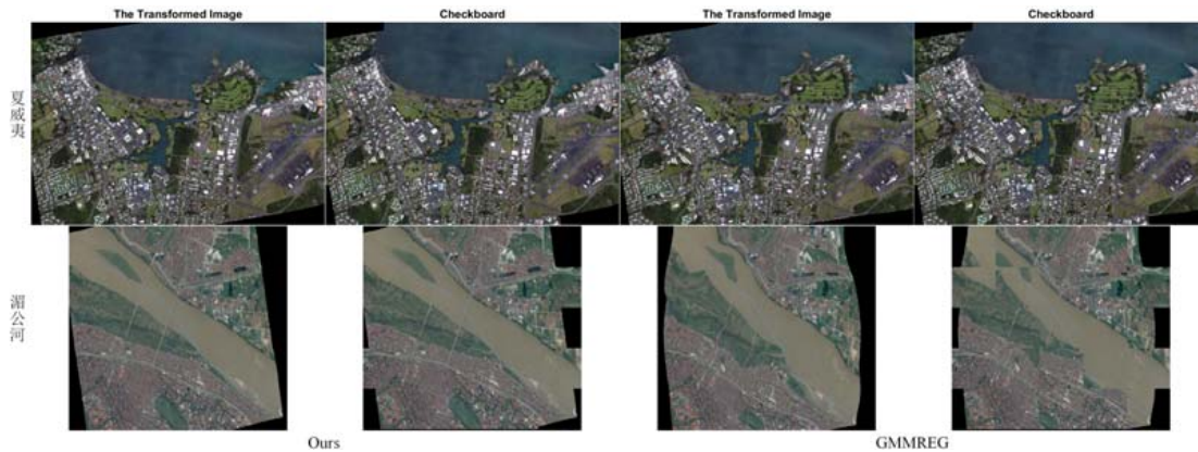
Fig.11 Remote sensing image registration results of our algorithm and GMMREG
