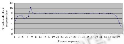
Fig.2 Relationship between response time and load
