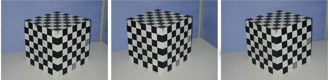
Fig.3 Three calibration object images used for experiment
