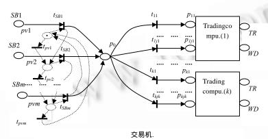
Fig.1 A subnet model of the prepositional computer static processing system
