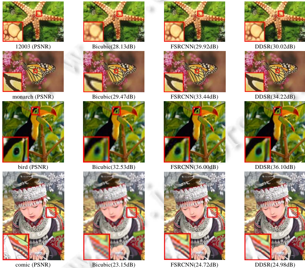
Fig.7 The reconstruction images (X3) of different image super-resolution methods
