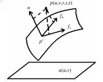
Fig.3 Projecting points to the B-spline base surface
