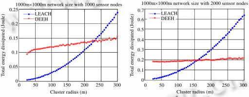
Fig.3 Total energy dissipated of clustering formation for 1000×1000m<sup>2</sup> with 1000 and 2000 nodes
