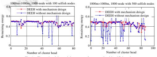
Fig.4 Cluster heads' remaining energy for network with selfish nodes
