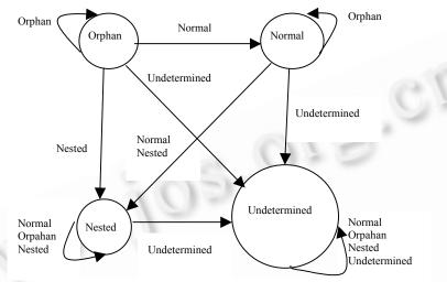
Fig.3 State transition model for nesting type combination
