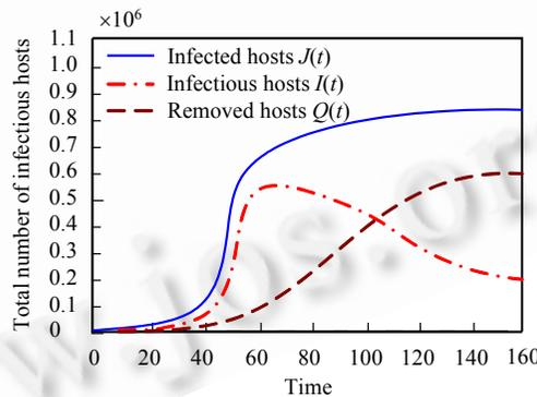
Fig.5 Internet worm propagation trend in two-factor model
