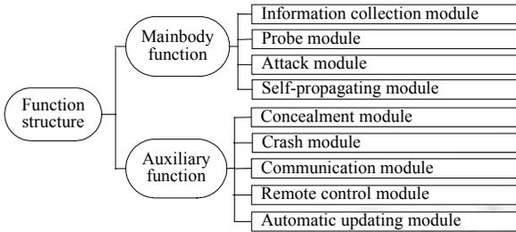
Fig.1 Function c structure of Internet worms
