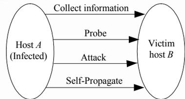
Fig.2 Execute mechanism of Internet worms
