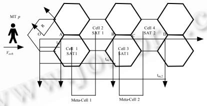
Fig.1 Meta-Cell architecture in LEO networks
