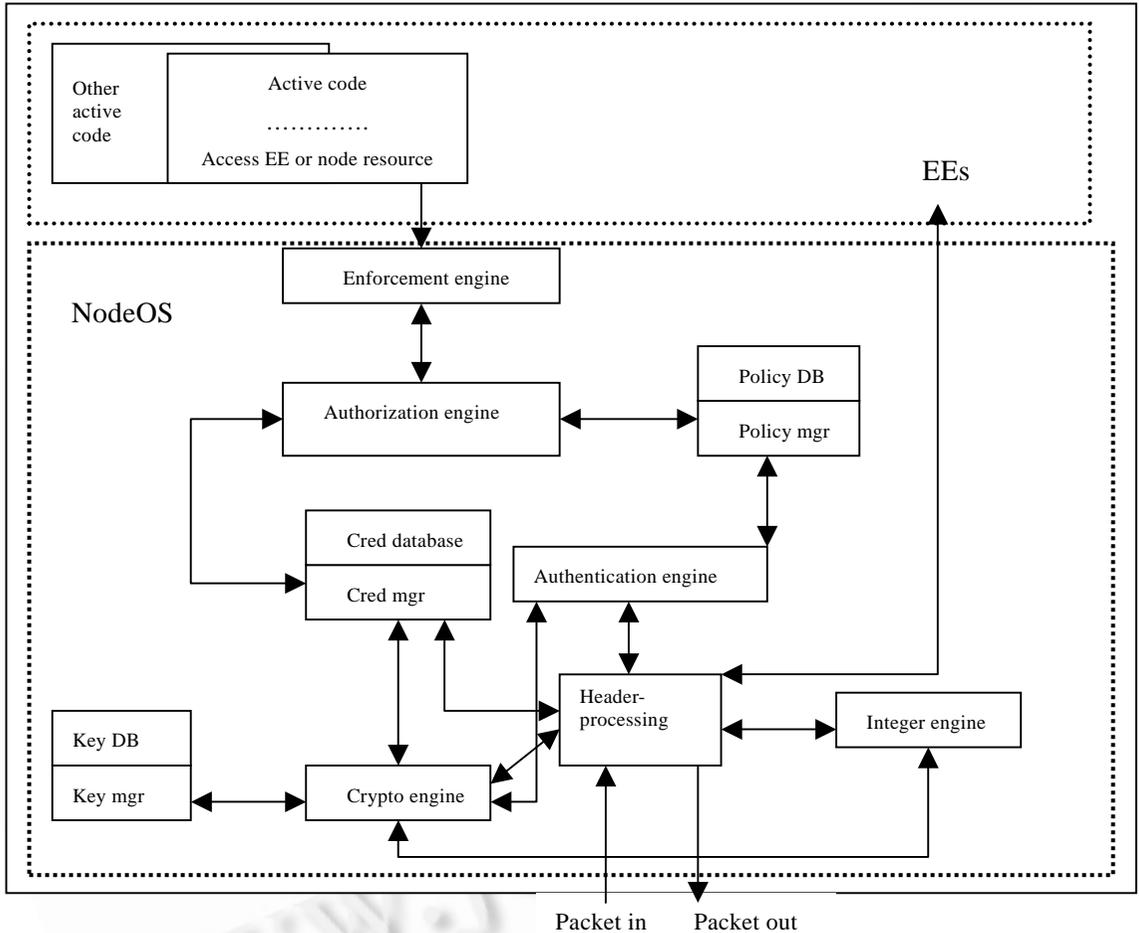
Fig.3 Secure system architecture
