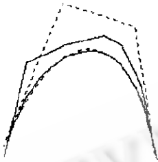
Fig. 1 Reduction of the degree 6 Bézier curve
