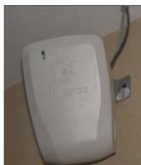
(a) The UWB sensor installed on the wall
