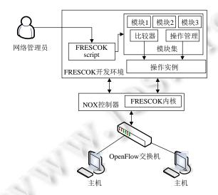
Fig.10 Abnormal traffic detection framework of FRESCO<sup>[37]</sup> 图 10 FRESCO 异常流量监测框架<sup>[37]</sup>
