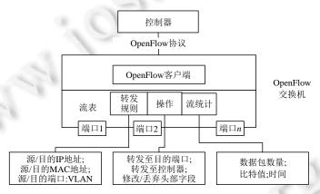
Fig.2 Communication between the controller and the forwarding devices via OpenFlow protocol<sup>[11]</sup> 图 2 控制器与转发单元之间通过 OpenFlow 协议<sup>[11]</sup>进行通信
