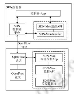
Fig.6 Abnormal traffic detection framework of SDN-Mon<sup>[31]</sup> 图 6 SDN-Mon 异常流量检测框架[31]
