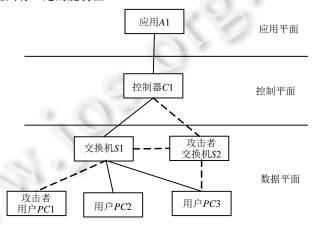
Fig.3 Abnormal flow attacks on the data plane 图 3 数据平面的异常流量攻击
