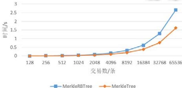
Fig.7 MerkleRBTree and MerkleTree build cost comparison
