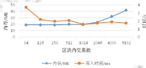
Fig.8 Impact of block size on memory and write time
