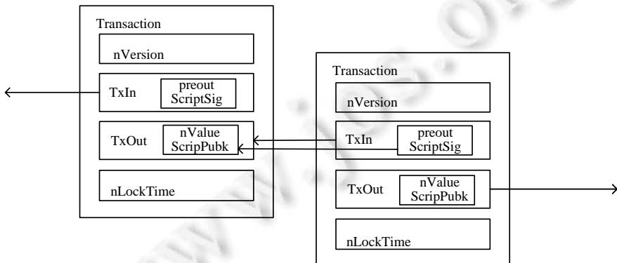
Fig.3 Transaction structure diagram
