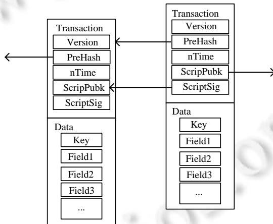
Fig.4 Database-oriented transaction structure
