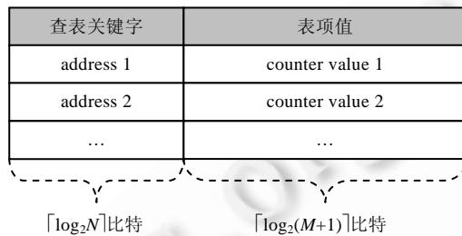
Fig.1 Structure of overflow table
