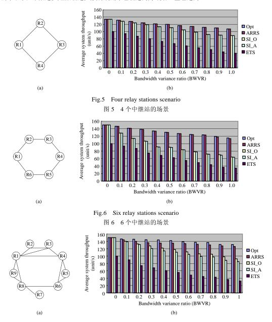
Fig.7 Nine relay stations scenario 图 7 9 个中继站的场景
