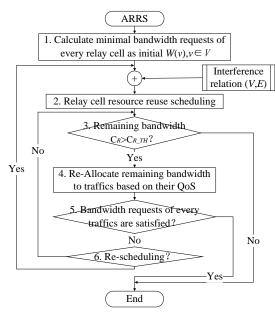
Fig.3 ARRS algorithm flowchart 图 3 ARRS 算法流程图
