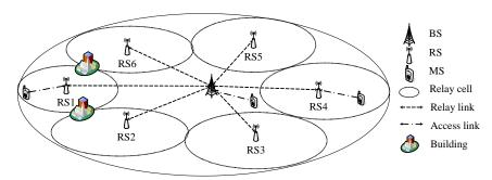
Fig.1 Multihop relay wireless network 图 1 无线多跳中继网络
