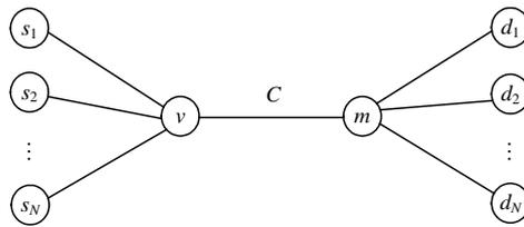
Fig.1 The model in most previous buffer sizing works
