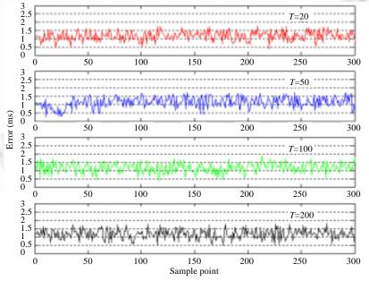
Fig.8 The impact of sampling cycle on synchronization error 图 8 采样周期对同步误差的影响
