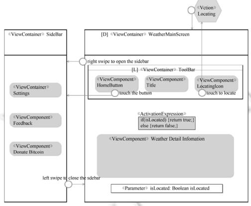
Fig.2 A part of IFML model for Good Weather
