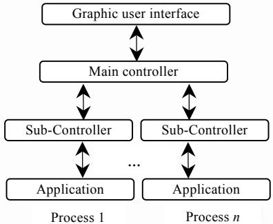
Fig.2 Architecture of XBUSTER
