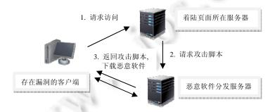
Fig.1 Typical process of drive-by download attack 图 1 典型网页木马攻击流程
